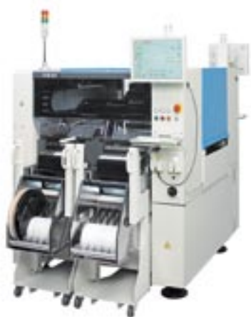
YS12 Compact high-speed modular surface mounter
