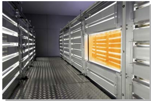
Yamaha High-efficiency Bio Reactor — a photosynthesis device developed for low-cost mass cultivation of microalgae
